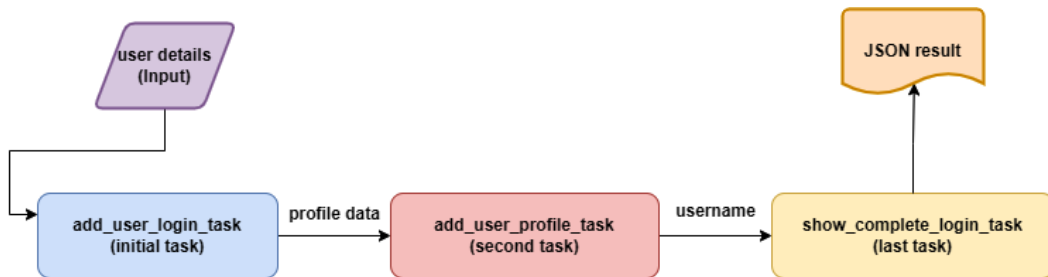
Figure 8.1 – Task signatures in a chain operation
