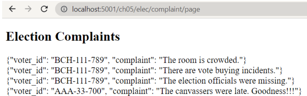
Figure 5.5 – An SSE client page rendering pushed data from Redis
